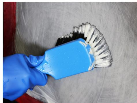
**Top tip:** Applying a 'stain preventer gel' to the screen immediately after printing can make cleaning much easier.
