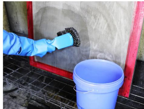
**Fused Acetate stains** - These are easily recognisable as a lightly coloured, translucent residue left on the screen where the stencil was. These stains can be removed using a low caustic haze remover such as Autokleen Plus activated with Autosolve Industrial AF Screen Wash.
