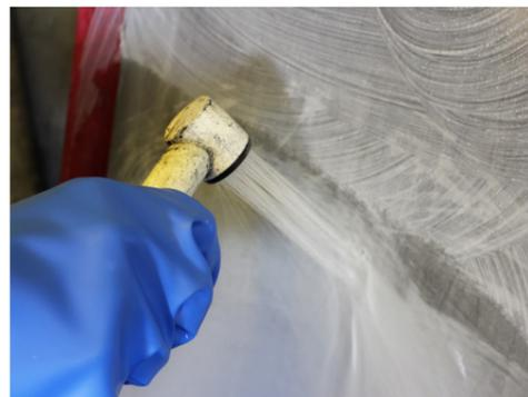
**Ink staining of the mesh fibres** - Some inks will actually dye polyester threads during printing. If this does happen the stain can only be removed with a very strong caustic haze remover, such as Autohaze. Although this type of stain does not reduce the mesh opening diameter it can cause problems during the exposure of subsequent stencils due to differential UV light absorption.
